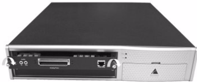
Figure 4. Access board installation
